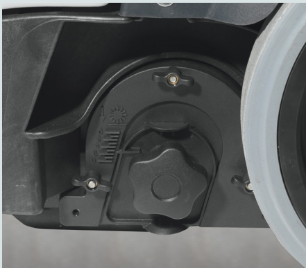
The main and side brushes are adjustable to ensure perfect pressure on the floor at all times and in all conditions.
