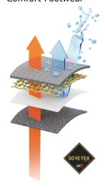
The GORE-TEX membrane prevents water from entering into the shoe, but still allows your feet to "breathe". This technology provides ideal climate comfort for all outdoor activities, even in the harshest weather conditions. All components of the shoe construction are precisely attuned to one another and are subject to constant quality controls.
